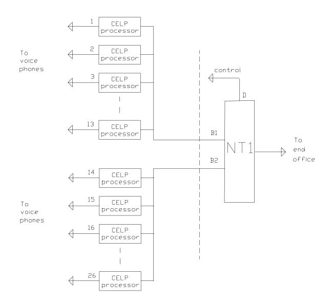
Figure 1 - Proposed NT26 The dashed line represents the standard T point. Components at right are standard ISDN chips.
